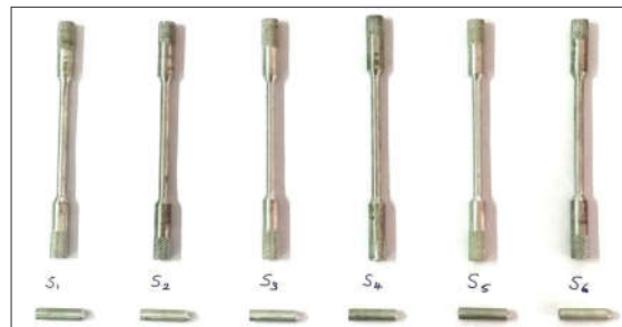
Fig. 3. Tensile and wear test samples
