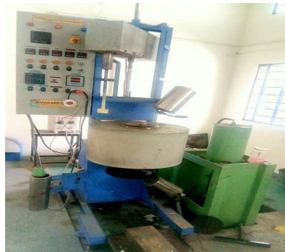
Fig. 1. Squeeze casting machine setup
