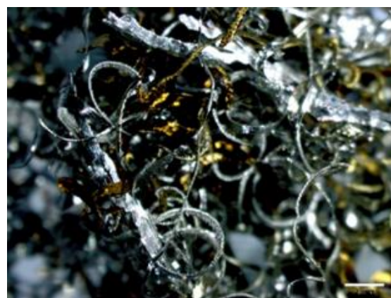
Fig. 1. AA 7075 swarf produced from the machining process
