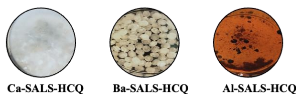
Fig. 7. Stability of beads PBS (pH 7.4) after 1 hr
