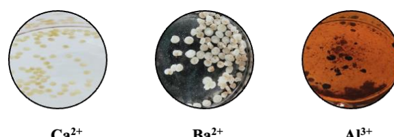
Fig. 5. Stability of beads in SGF (pH 1.2) after 1 hr
