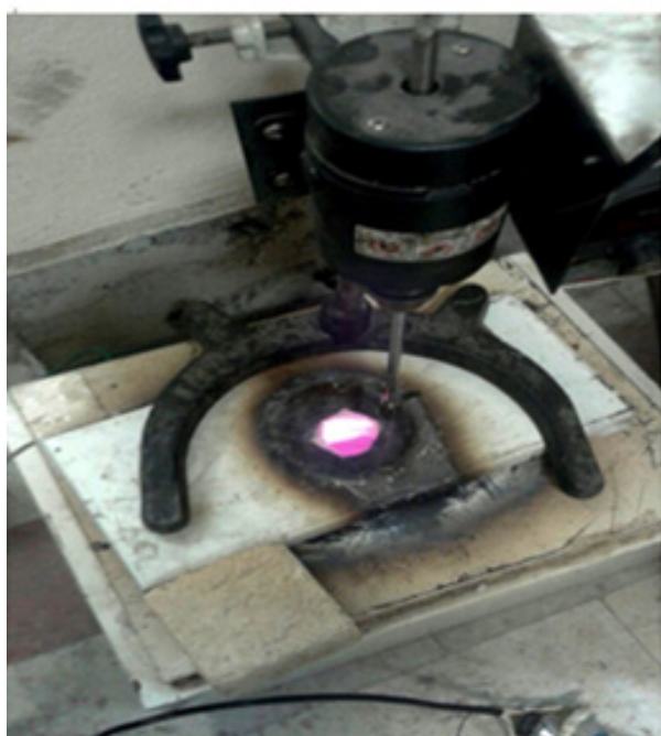
Fig. 4. a) Ultrasonic probe and (b) mechanical stirrer and ultrasonic device.
