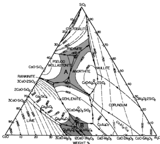
Fig. 1. Low melting temperature region A and B in \text{CaO-Al}_2\text{O}_3\text{-SiO}_2 system [4].
