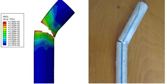
**Fig. 10.** Fractured AA 6063-T6 tube after (a) simulation and (b) experimental bending test at a bending radius of 32.5 mm.
