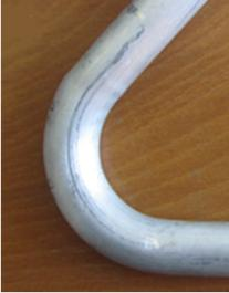
**Fig. 6.** Simulation and experimental bending results of AA6063-O tubes for a bending radius of 40 mm and a bending angle of 135°.
