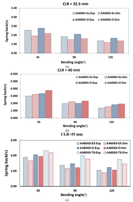
**Fig. 17.** Comparison of experimental and simulation results of spring-back for A6063-Ex, AA6063-O, and AA6063-T6 tubes at the bending radius of (a) 32, (b) 40, and (c) 55 mm.
