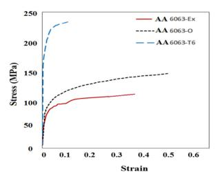
Fig. 3. Stress-strain curves of AA6063 with three different conditions.
