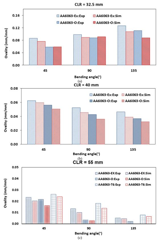
**Fig. 15.** Comparison of experimental and simulation ovality results of AA6063-Ex, AA6063-O, and AA6063-T6 tubes at a bending radius of (a) 32.5, (b) 40, and (c) 55 mm.
