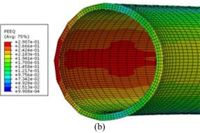
**Fig. 13.** Wall-thinning and ovality in the middle part of the tube in (a) experimental and (b) simulation results.
