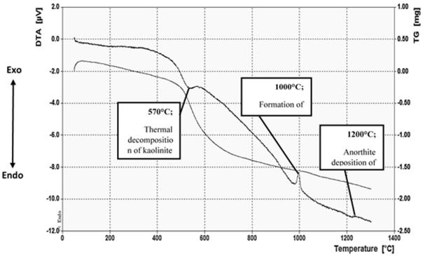
Fig. 2. DTA and TGA analyses for sample A50
