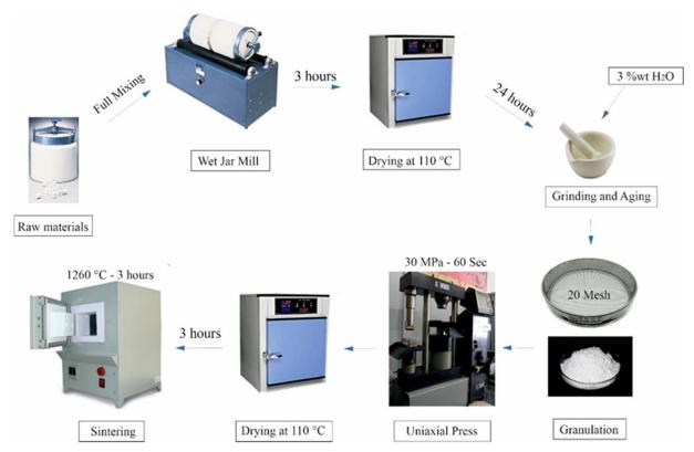
Fig. 1. Manufacturing steps of the produced bodies
